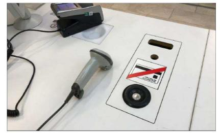
Figure 2: Magnetic hard label remover
