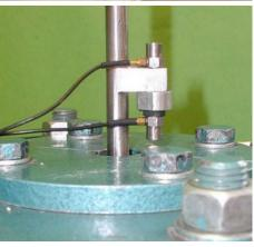
Comparison measurements of piezoelectric vibration transducers and a LASER vibrometer
