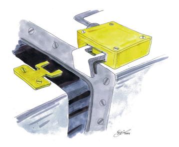
Position switch for detection of the door position, defeated by means of a substitute actuator
