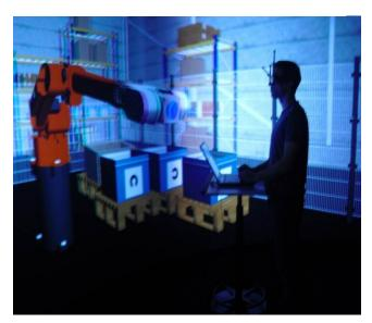
A test subject working with a virtual collaborative robot in the IFA's SUTAVE laboratory
