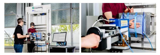
Figure 3. Algometer that produces clamping loads (quasi-static contacts)
